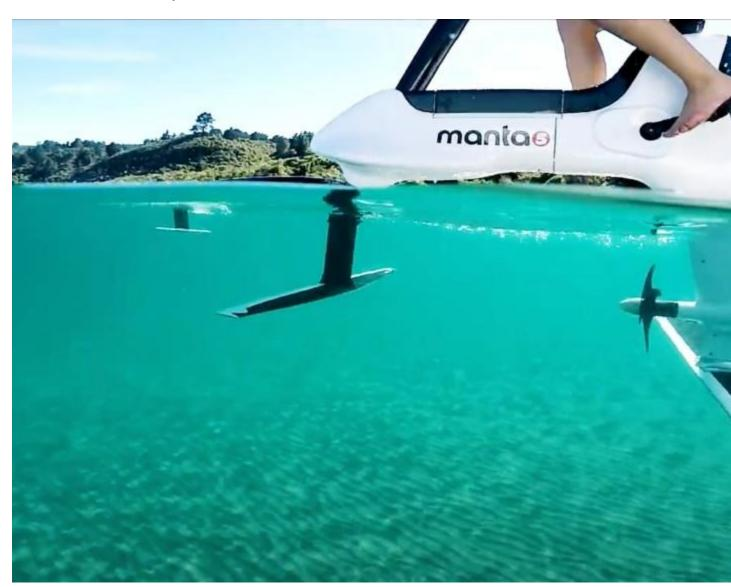
The foils on the Manta5 hydrofoiler provide stability, while its electric motor can push its non-pedaling speed up to 12 mph. Courtesy Manta5
