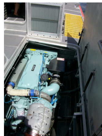
This is one of the twin 800+ h. p. engines that can power the boat to over 40 knots.
