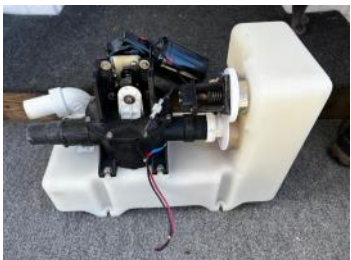
Pump body assembly. Duckbill valves are located inside the black tubes on each side
