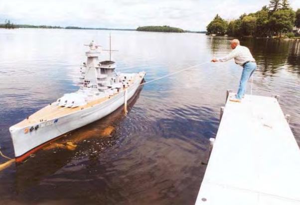
The model is scratch built using 14" bass wood strips & then covered w/fiberglass. Estimated weight: 700 lbs. The beam is 52" The length is about 30' It can carry 2 persons. The model is powered by a 15 hp outboard engine located under rear gun turret.
