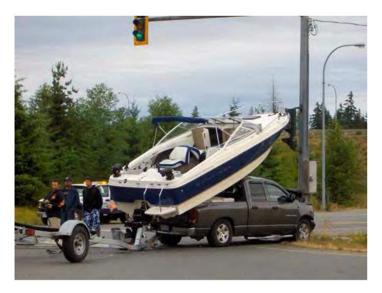
VEs also check the trailer when the VSC is conducted on the trailer. If we had done this boat, it might still be on the trailer. You will note that both the truck and boat hit the power pole.
